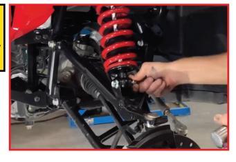
Loosen OEM upper preload ring from OEM lower preload ring. Use flathead screwdriver and hammer.
