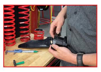
Install OEM spring divider with long end pointing up into the new ZBROZ Tender Spring. Place the OEM Reducer on top as shown.
