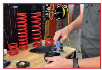
To help you cut a straight line make a few marks around the retainer and then run black electrical tape along your marks. Using a hack saw or other cutting device cut the 2" off the at your cut marks.
