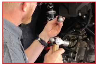
Rotate OEM spring stack and preload ring counter clockwise to the top of the threaded shock body or until springs are loose & free.
