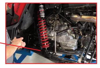
Loosen the top preload nut by using a flathead screwdriver as shown and knocking it counterclockwise. Lossen enough so that the nut is out of the way.
